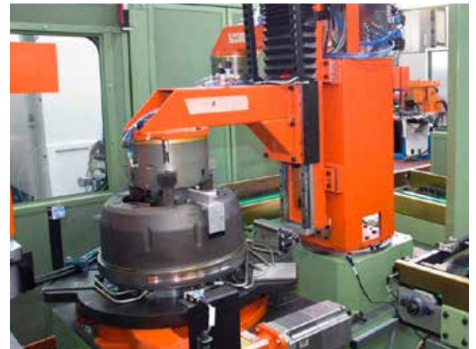
Equilibratura di tamburi camion Truck drum balancing
